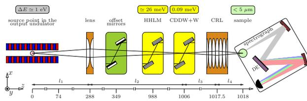
Figure 3: Main optical components of the proposed UHRIX instrument at the SASE2-undulator beamline of the European XFEL shown schematically together with the output undulator. Optical components are presented as pictographs at certain distances from the source position measured at the beam waist in the SASE2 undulator, which is at 74 m from undulator's downstream end. See text for descriptions.
