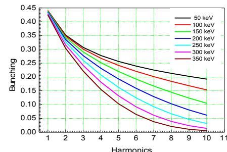
Figure 1: Bunching factor for HGHG with different initial slice energy spreads.
