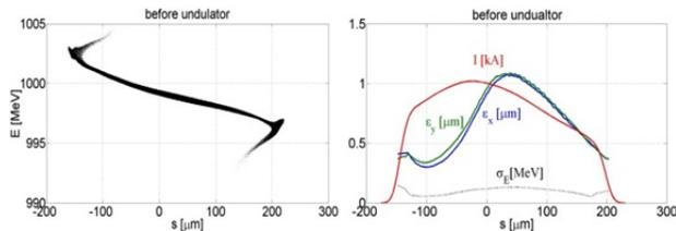
Figure 2: Bunch properties before the modulator for 1.0 nC case. Longitudinal phase space (left), Current profile, slice emittances and slice energy spread (right).
