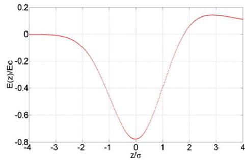
Figure 4: Normalized longitudinal field of an ultra-relativistic thin Gaussian bunch in circular motion.
