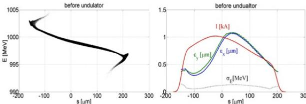
Figure 2: Bunch properties before the modulator for 1.0 nC case. Longitudinal phase space (left), Current profile, slice emittances and slice energy spread (right).
