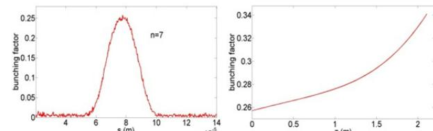
Figure 6: Bunching factor before the radiator (left) and bunching distribution along the radiator (right).
