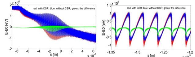
Figure 5: Density modulation and CSR impact on microbunches in the dispersive chicane.
