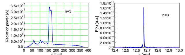
Figure 11: Radiation power at the exit of the radiator (left) and the spectrum (right).
