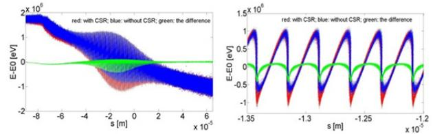
Figure 5: Density modulation and CSR impact on microbunches in the dispersive chicane.
