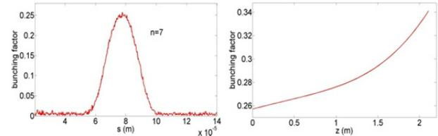
Figure 6: Bunching factor before the radiator (left) and bunching distribution along the radiator (right).
