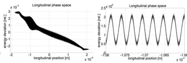
Figure 3: Longitudinal phase space after the modulator.
