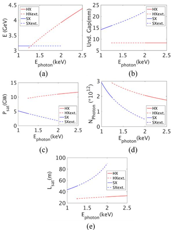
Figure 2: Blue (red) line indicates the existing SXR (HXR) undulator line. Solid (dashed) line means provided (vacant) photon energy region (a) Electron beam energy (b) Undulator gap (c) Saturation power (d) Number of photons (e) Saturation length.
