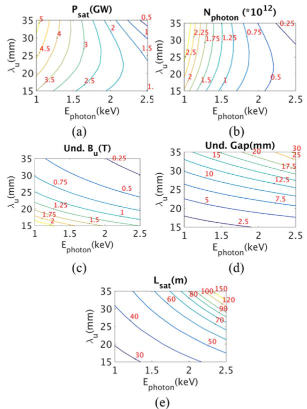
Figure 3: Contour graphs vs. undulator period and resonance photon energy in 3.15 GeV branch linac (a) Saturation power (b) Number of photons (c) Undulator peak magnetic field (d) Undulator gap (e) Saturation length.
