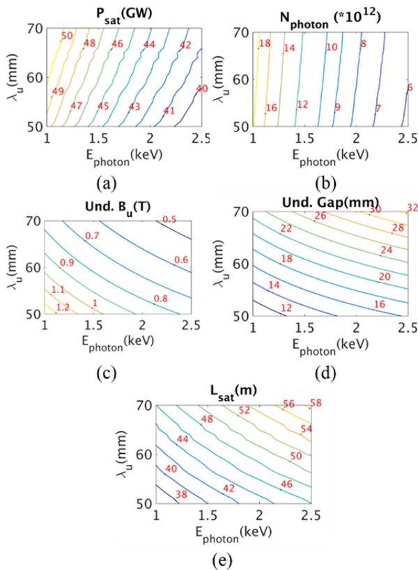
Figure 4: Contour graphs vs. undulator period and resonance photon energy in 10 GeV main linac (a) Saturation power (b) Number of photons (c) Undulator peak magnetic field (d) Undulator gap (e) Saturation length.
