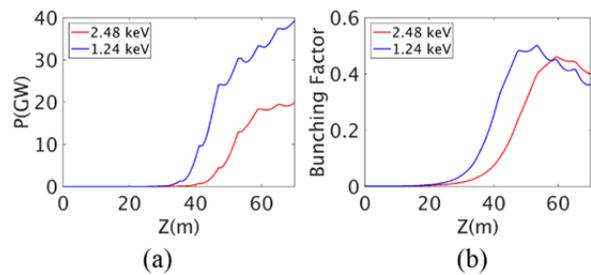
Figure 5: SASE simulation results with non-tapering. Blue (red) line indicates 1.24 (2.48) keV photon energy. (a) Radiation power (b) Bunching factor.
