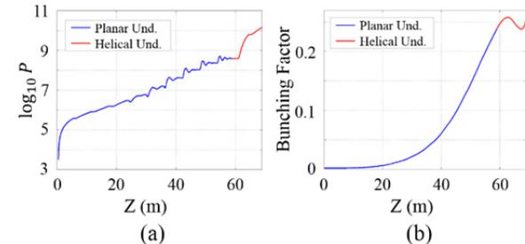
Figure 6: Polarization control with EPU simulation results. Blue (red) line indicates planar (helical) undulator output. (a) Logarithmic radiation power (b) Bunching factor.
