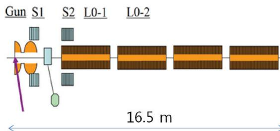
Figure 1: Layout of the injector lattice for the Soft X-ray FEL design.
