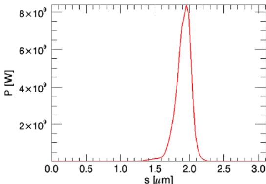
Figure 7: Temporal power profile at \$z = 30\$ m.
