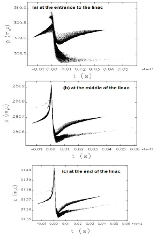
Figure 3: Longitudinal phase space distribution in the linac.
