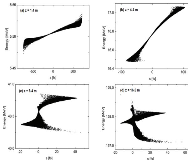
Figure 2: Longitudinal phase space distribution in the injector.
