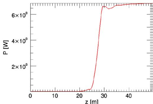
Figure 6: Average radiation power along the undulator position \$z\$.
