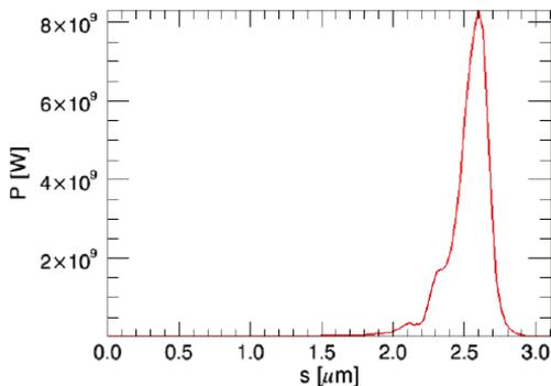
Figure 8: Temporal power profile at \$z = 50\$ m.
