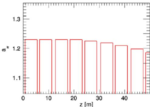
Figure 5: Stepwise tapering of the undulator parameter for the soft XFEL simulation.
