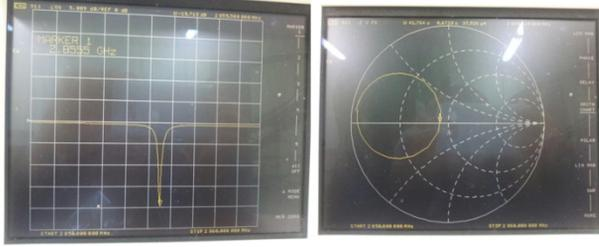
Figure 4: Cold test results of S11 parameter (left) and smith chart (right) of the deflecting cavity.
