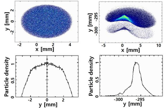
(a) Without RF field in the cavity (b) With RF field in the cavity
