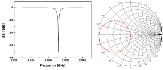
Figure 3: S11 parameter (left) and Smith chart (right) of the simulation of the deflecting cavity.
