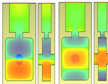
Figure 2: Electric field (left) and magnetic field (right) distribution of  $TM_{120}$  mode in the deflecting cavity.
