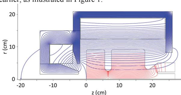
Figure 1: MaRIE photoinjector, showing RF cavity based on the PITZ design (red field contours) with a new solenoid design (blue contours).
