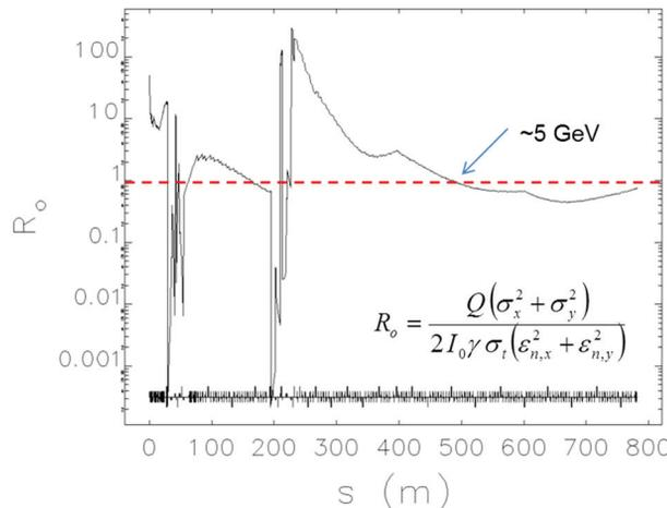
Figure 3: Space charge impact parameter along the MaRIE linac.  $R_0 > (<) 1$  implies space-charge (emittance) dominated beam dynamics.
