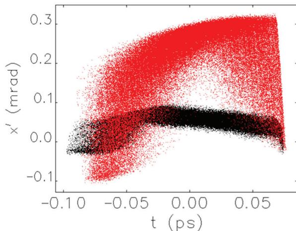
Figure 2: **elegant** [20] simulation of  $t$ - $x'$  phase space for a 57:1 compression ratio with a single (red) and dual (black) chicane compressor.
