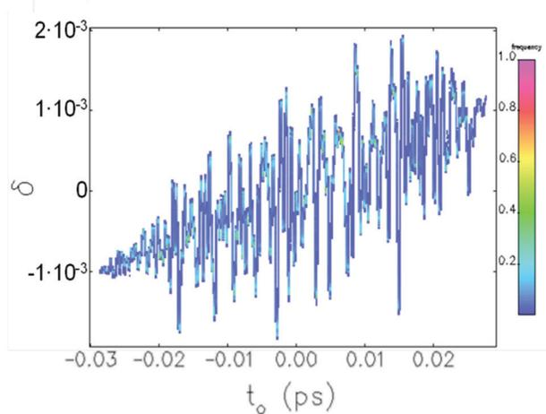
Figure 4: Longitudinal phase space at the end of the MaRIE linac.
