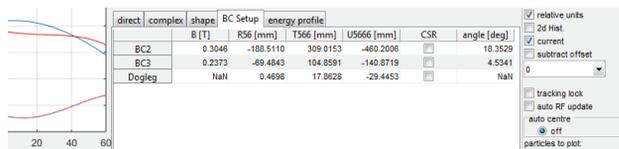
Figure 3: An example of the setup of dispersive sections. While the chicanes can be adjusted by the field, or bending angle, the dogleg or collimator sections are represented by the matrix elements. CSR calculations can be activated for each chicane individually.
