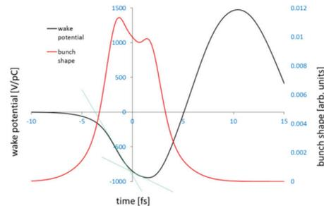
Figure 7: The shape of the experimentally measured two horn bunch (red line) and the corresponding wake potential (black line). Light green lines show two slopes.
