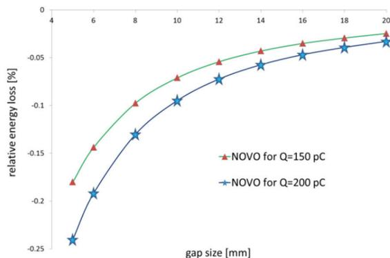
Figure 8: Relative energy loss of a bunch with a charge of 150 pC (green line with red triangles) and 200 pC (black line with blue stars).
