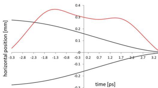
Figure 9: Horizontal position of the bunch boundary particles (black lines) downstream of the dechirper for a bunch charge of 200 pC. The red line shows the bunch charge distribution.
