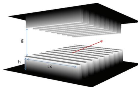
Figure 1: A schematic drawing of a dechirper. The red line shows a bunch trajectory.
