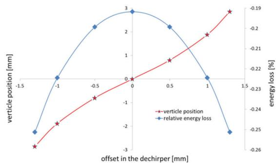
Figure 10: Vertical position of the bunch downstream of the dechirper (red line with red stars) and energy loss (blue line with diamonds) as a function of the vertical offset in the dechirper for a gap of 6 mm. The bunch charge is 200 pC.
