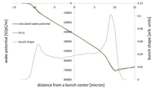
Figure 4: Comparison of the wake potential calculated using a computer code (red line) and calculated using a Green's function (green line) for a two horn bunch passing a dechirper with a 1 mm gap.
