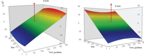
Figure 5: Integrated vertical and horizontal force distribution when a bunch trajectory lies in the center, between the jaws and in the middle of the diaphragms of the dechirper. Red arrows show the bunch trajectory.
