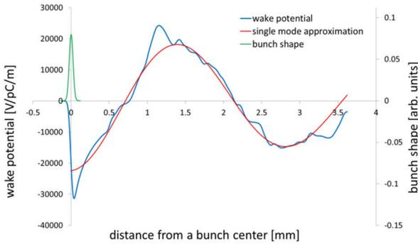
Figure 2: Wake potential (a blue line) of a 25 micron bunch passing through a 2 m rectangular corrugated structure with a full gap of 1.4 mm. The red line shows a single mode approximation. The green line shows the bunch charge distribution.
