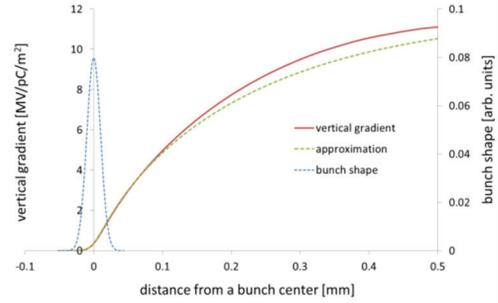
Figure 6: Vertical gradient of the transverse wake fields of a 10 micron bunch (red line), approximation of the vertical gradient (green dashed line) and bunch charge distribution (dotted blue line).
