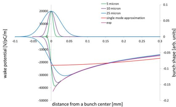
Figure 3: Wake potential of a 5 micron bunch (green line), 10 micron (magenta line) and 25 micron (blue line). The red line shows a single mode approximation and the pink line show the exponential function.
