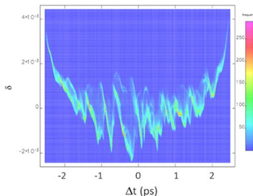
Figure 4: Electron beam longitudinal phase space after one turn in RIBS. Copyright of American Physical Society [3].
