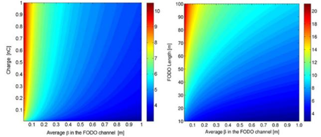
Figure 1: IBS-induced rms energy spread in keV, in the  $(\beta, Q)$  space for  $L = 30$  m (left), and in the  $(\beta, L)$  space for  $Q = 500$  pC. Both plots are for a beam energy of 150 MeV. The beam transverse emittances and the bunch duration are scaled with  $Q$  as explained in the text. Notice that the colour scale is different in the two plots. Copyright of American Physical Society (APS) [3].
