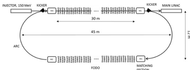
Figure 3: Schematic layout of the recirculating IBS beam line (not to scale). Copyright of American Physical Society [3].
