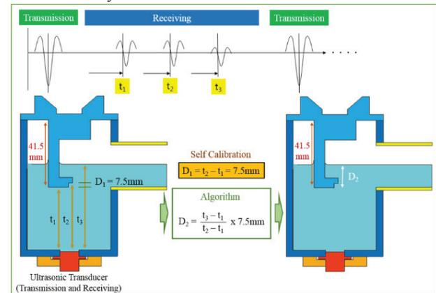
Figure 8: Measuring the height of water surface using ultrasonic waves.
