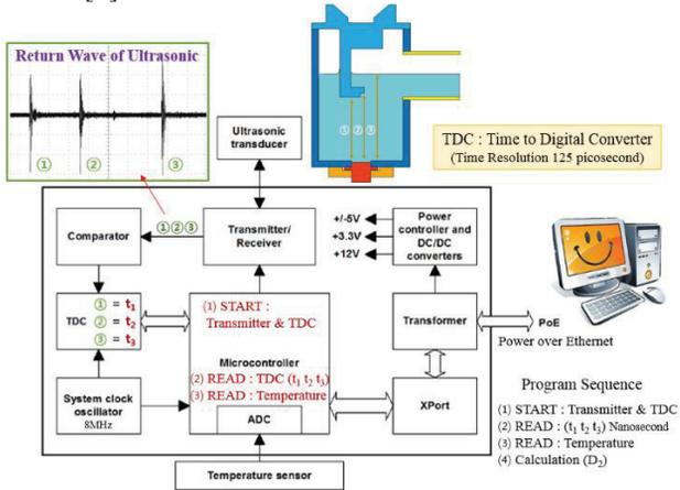
Figure 9: Block diagram of the ULSE Electronics.
