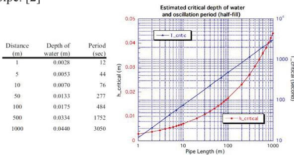
Figure 5: The critical (optimum) depth of water and the period of oscillation for different lengths of pipes in a half-filled system.
