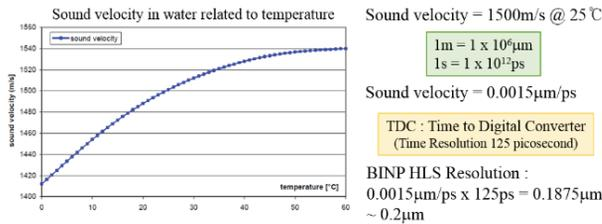
Figure 10: Resolution for measuring the distance of BINP HLS.
