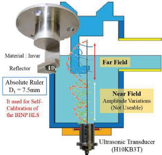
Figure 7: The HLS measurement concept using an ultrasonic transducer.
