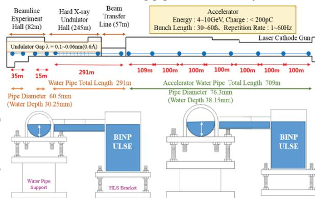
Figure 6: The length and diameter of a water pipe.
