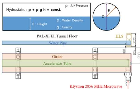
Figure 4: The position of water pipes inside the accelerator tunnel.
