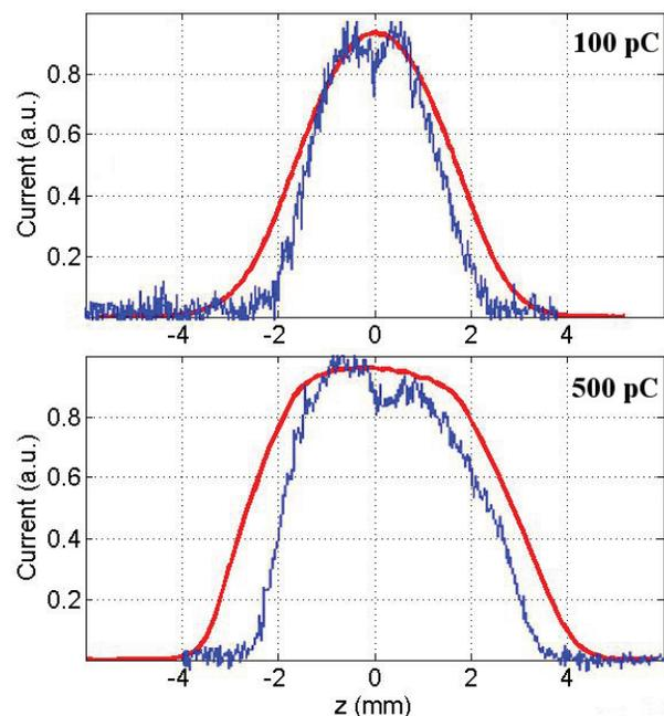
Figure 5: Longitudinal profiles of 100 pC (top) and 500 pC (bottom) bunches after the TDS. The smooth red curves are ASTRA simulations assuming a 11.5 ps (FWHM) long Gaussian photocathode laser pulse, the blue curves are TDS measurements.
