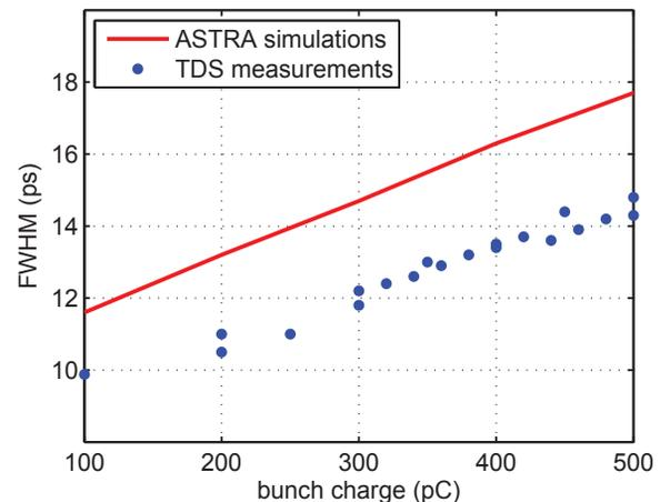
Figure 4: FWHM bunch lengths, measured and simulated, for bunch charges between 100 and 500 pC. The booster phase was tuned for maximum mean momentum gain.
