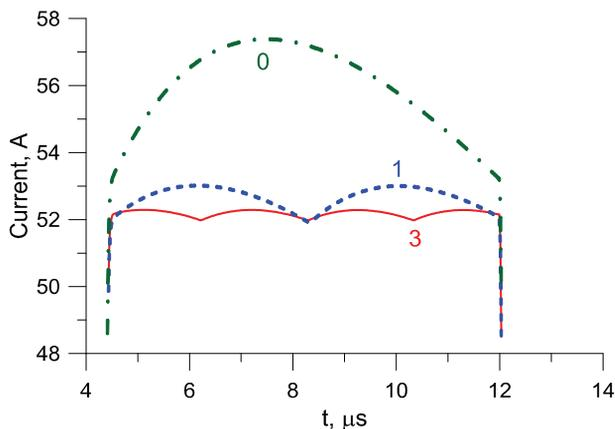
Figure 7. Current shape with different correctors.
