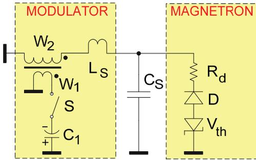
Figure 2: Modulator and magnetron equivalent circuit.
