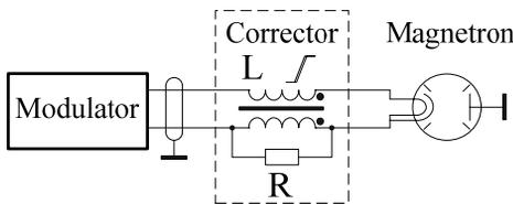
Figure 3. Simple corrector circuit.
