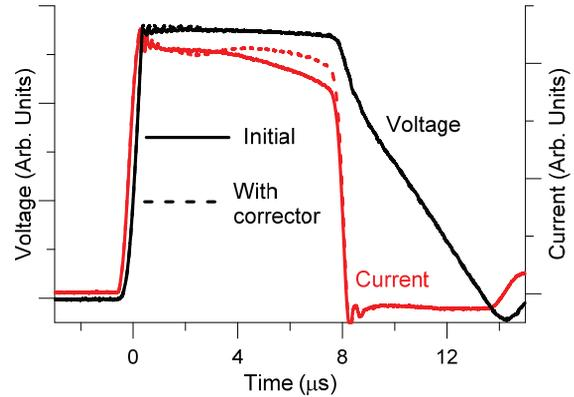
Figure 4. Current pulse shape modification.
