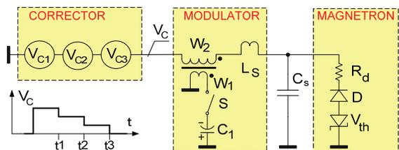
Figure 6. Modulator with a multi-cell corrector.
