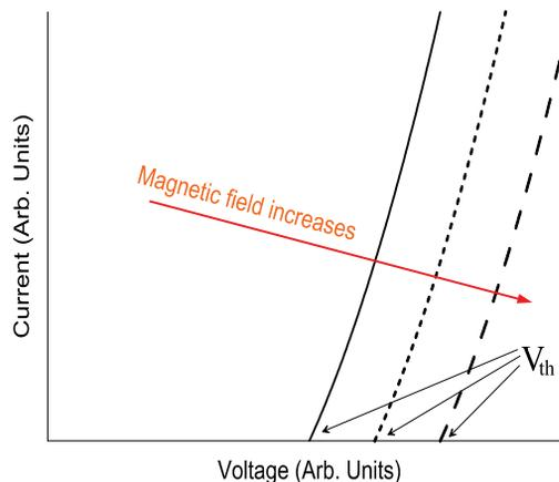
Figure 1: Volt –Ampere characteristic of a magnetron.
