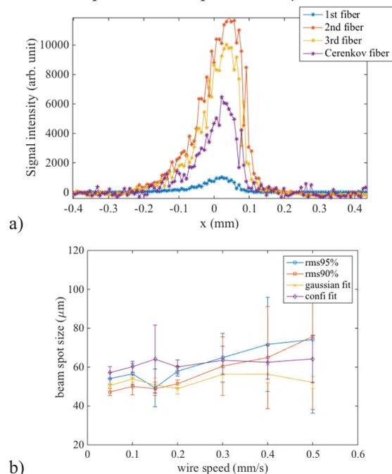
Figure 3: a) Horizontal beam profile acquired by the four monitors for the vertical 5- $\mu\text{m}$  wire scanning at 0.1mm/s. b) Horizontal beam size ( $\sigma_x$ ) versus the wire speed obtained by processing in four different ways the profile measured with the second fiber.
