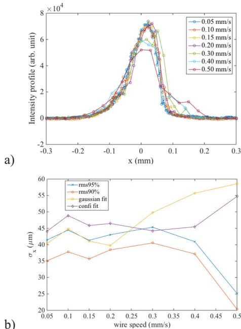
Figure 4: a) Horizontal profile integrated over six profiles acquired with the second fiber at different wire speed; b)  $\sigma_x$  obtained with the four methods as a function of the wire speed. At wire speed = 0.5mm/s, the measurements are not reliable due to the poor resolution in sampling the beam profile.
