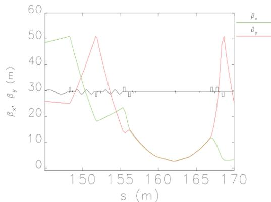
Figure 2: The horizontal and vertical  $\beta$ -function along the straight path at the end of the linac. The origin ( $s=0\text{m}$ ) of the horizontal axis corresponds to the electron source, i.e. the photo-cathode plate.
