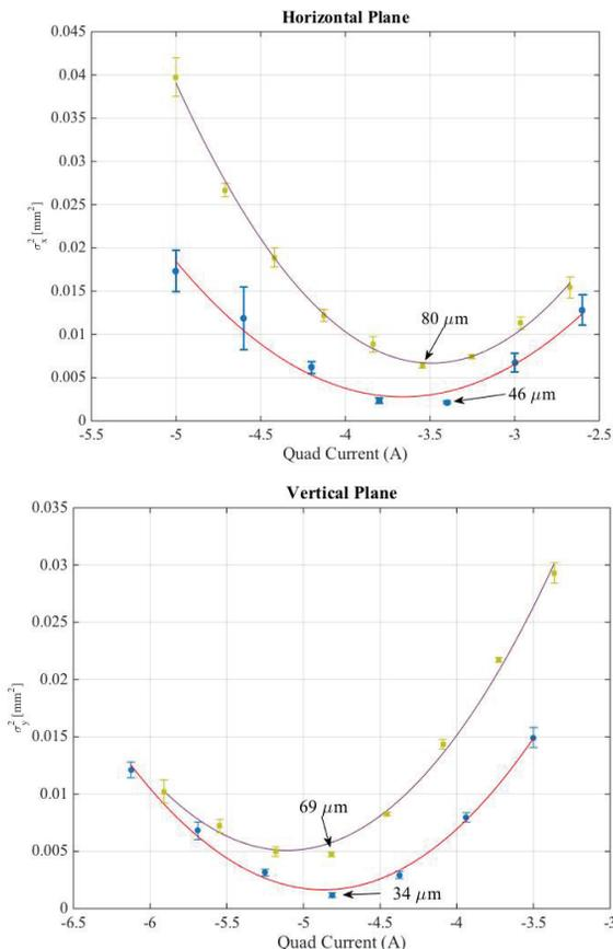
Figure 5: Horizontal (top) and Vertical (bottom) beam spot size versus the quadrupole Q<sub>2</sub> current measured by the WS device (blue circles data and red line) and by the Sc<sub>2</sub> (yellow squares data and purple line). The horizontal profile was measured with the 5- $\mu$ m wire, while the vertical one with the 13- $\mu$ m wire.
