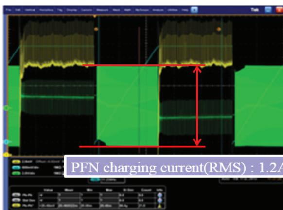
Figure 5: PFN charging current.
