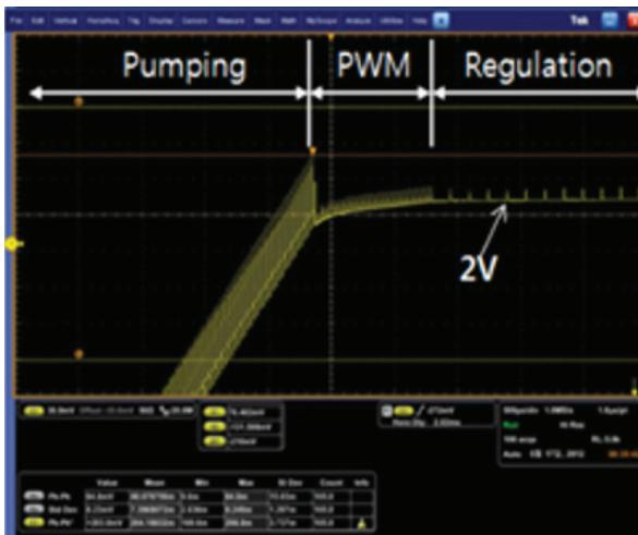
Figure 6: Current of PFN charging voltage.
