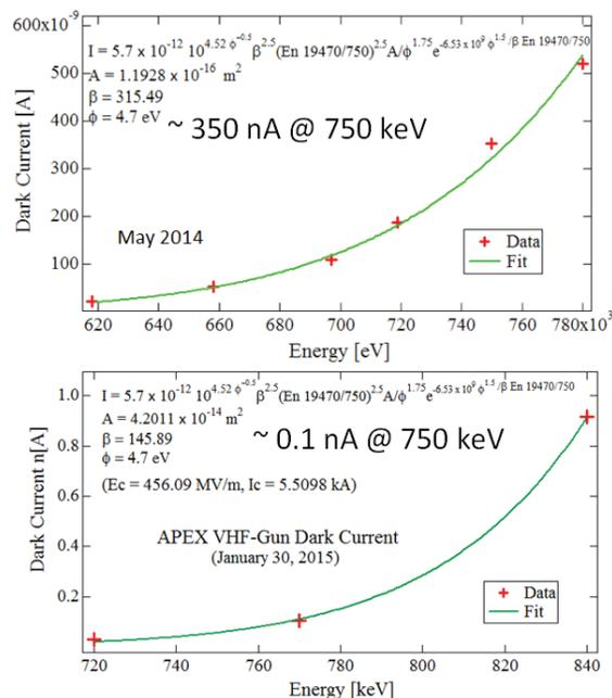
Figure 10: Dark-current Fowler-Nordheim analysis before (top) and after (bottom) the cleaning/re-polishing operation.
