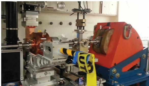
Figure 5: Part of the Phase-II diagnostics beamline. The 1.3-GHz single-cell transverse deflecting copper cavity is visible in the left of the picture followed downstream by the large orange spectrometer (vertical) bending magnet.
