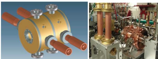
Figure 2. Left: APEX buncher CAD view. Right: a picture of the buncher installed in the Phase-II beamline.
