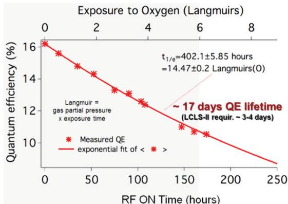
Figure 9: Cs<sub>2</sub>Te QE vs. time and integrated Oxygen exposure.
