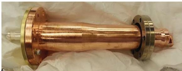
Figure 3: APEX Buncher RF coupler.
