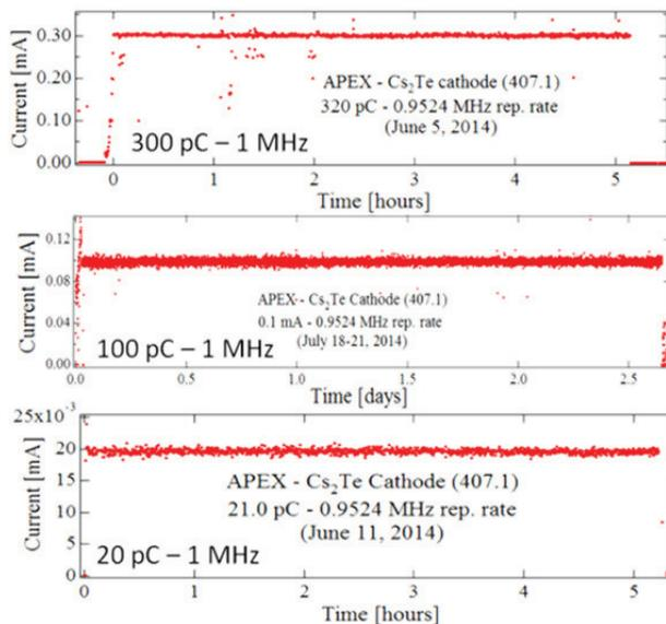
Figure 8: Example of constant current tests with Cs<sub>2</sub>Te.
