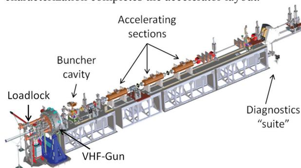
Figure 1: APEX Phase-II Layout.
