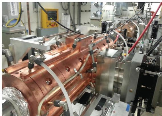
Figure 4: The modified AWA accelerating sections installed in the Phase-II beamline.
