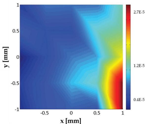
Figure 8: Quantum efficiency map of cathode at the UED beamline.
