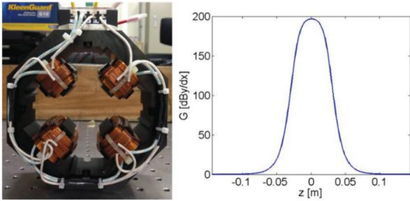
Figure 4: Photo and focusing field distribution of quadrupole lens.
