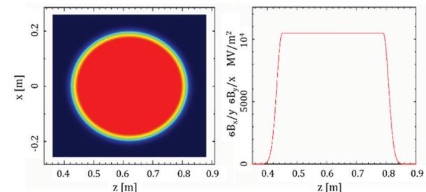
Figure 3: Magnetic field distribution of the 45-degree bending magnet.
