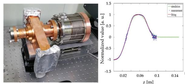
Figure 2: Photo of experimental setup for bead test and measured field distribution.
