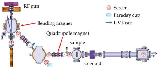
Figure 1: Schematic diagram of UED beamline at the KAERI and experimental setup.
