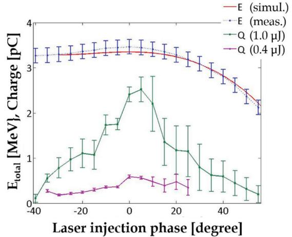
Figure 6: The measurement results of total energy and charge as function of a laser injection phase.
