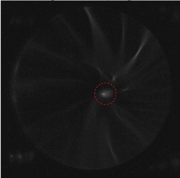
Figure 5: An electron beam image (red dot circle) with a dark current at the screen1.
