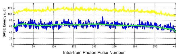
Figure 5: Pulse energy of 400 photon pulses in one train, pulse spacing 1 μs (1 MHz), photon wavelength 9.9 nm. Blue: Actual value, Green: Average, Yellow: Maximum.
