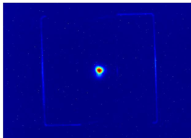
Figure 6: FLASH2 FEL radiation spot on a YAG screen. Photon wavelength 5 nm. The diffraction pattern is caused by a MCP mesh inserted upstream of the screen.
