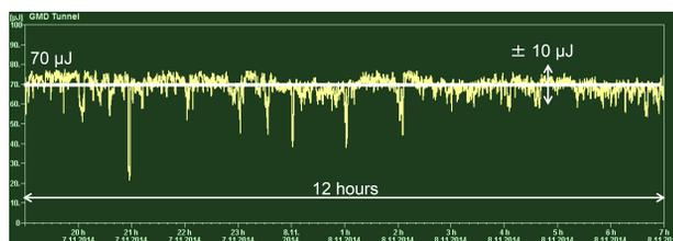
Figure 4: Average photon pulse energy during 12 hours of FEL radiation delivery. Photon wavelength 9.9 nm, 400 photon pulses per train, pulse train repetition rate 10 Hz, photon beamline aperture 3 mm.
