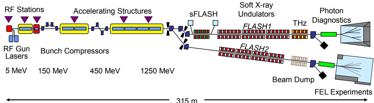
Figure 2: Layout of the FLASH facility (not to scale).
