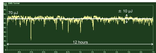
Figure 4: Average photon pulse energy during 12 hours of FEL radiation delivery. Photon wavelength 9.9 nm, 400 photon pulses per train, pulse train repetition rate 10 Hz, photon beamline aperture 3 mm.
