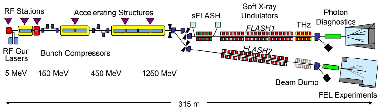
Figure 2: Layout of the FLASH facility (not to scale).
