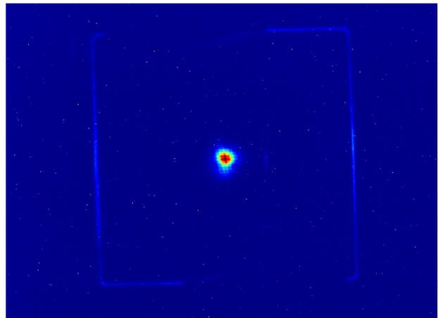
Figure 6: FLASH2 FEL radiation spot on a YAG screen. Photon wavelength 5 nm. The diffraction pattern is caused by a MCP mesh inserted upstream of the screen.
