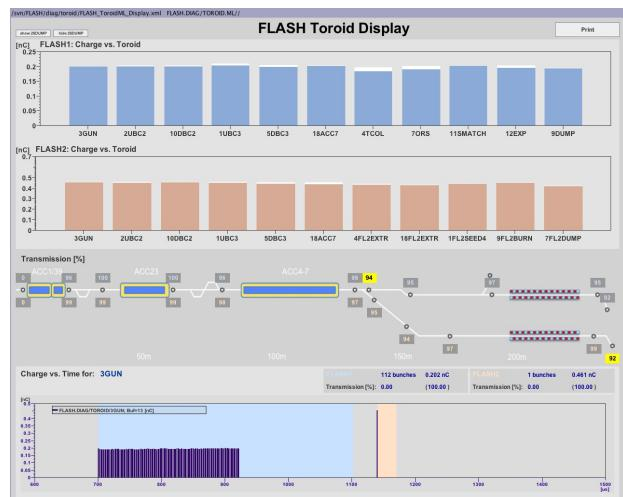
Figure 3: Example of simultaneous operation of FLASH1 and FLASH2. FLASH1 (blue): 112 electron bunches, bunch charge 0.2 nC. FLASH2 (salmon): single bunch with a charge of 0.4 nC.
