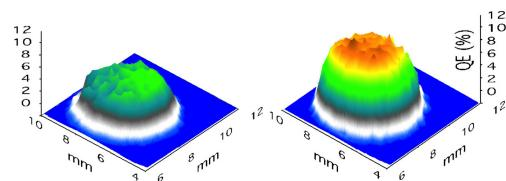
Figure 4: QE degradation after the 3-week shutdown and QE rejuvenation after few hours of gun operation at full power (from [7]).
