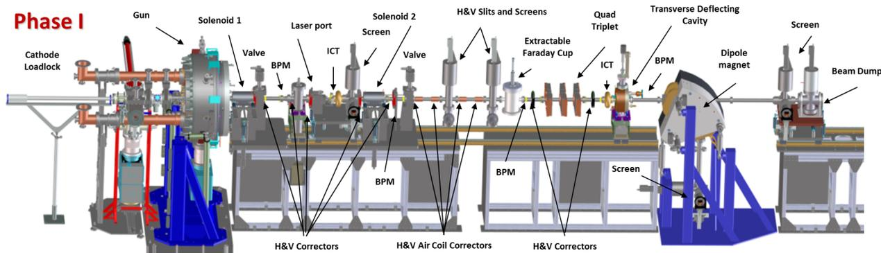
Figure 1: Cathode tested at APEX phase I beamline.
