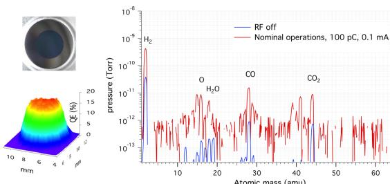
Figure 2: Left: image and QE map of the  $Cs_2Te$  cathode before operations (Courtesy of D. Sertore, INFN/LASA). Right: residual gas analysis in the APEX gun without RF power (blue) and during 0.1mA operations (red) (from [7]).
