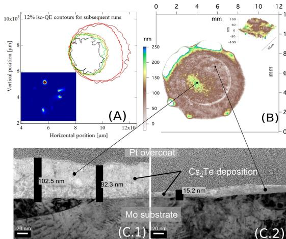
Figure 5: (A) Iso-QE contours during operations. The inset shows the asymmetric distribution of field-emitted particles, imaged at the beamline viewscreen. (B) Post-mortem interferometry on the cathode surface showing asymmetric erosion. The difference between peaks and valleys is at the level of film deposition thickness. (C.1-C.2) Post-mortem TEM measurements of the  $Cs_2Te$  layer in the peak and valley as shown in figure (from [7]).
