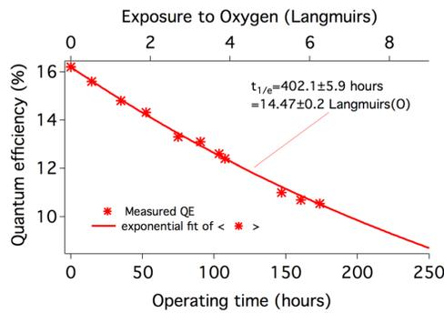
Figure 3: Exponential fit of QE as function of operational time and exposure to oxygen (from [7]).
