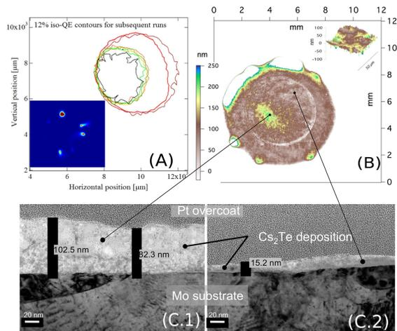
Figure 5: (A) Iso-QE lines during operations. The inset shows the asymmetric distribution of field-emitted particles, imaged at the beamline viewscreen. (B) Post-mortem interferometry on the cathode surface showing asymmetric erosion. The difference between peaks and valleys is at the level of film deposition thickness. (C.1-C.2) Post-mortem TEM measurements of the  $Cs_2Te$  layer in the peak and valley as shown in figure (from [7]).
