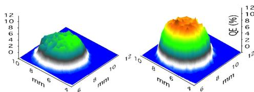
Figure 4: QE degradation after the 3-week shutdown and QE rejuvenation after few hours of gun operation at full power (from [7]).
