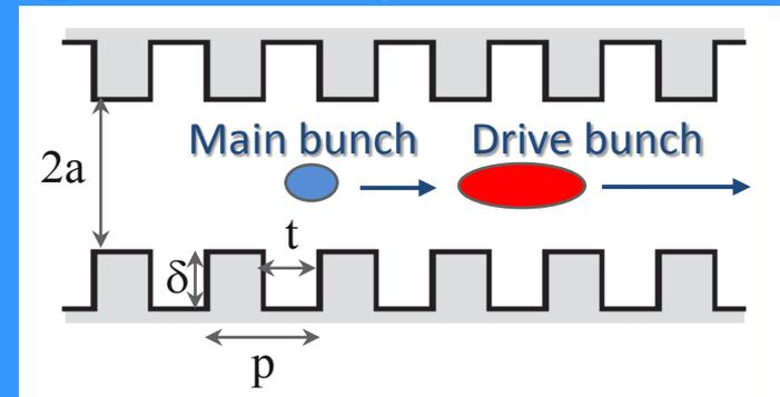
Drive and Main from the same source bunch → minimal timing jitter
