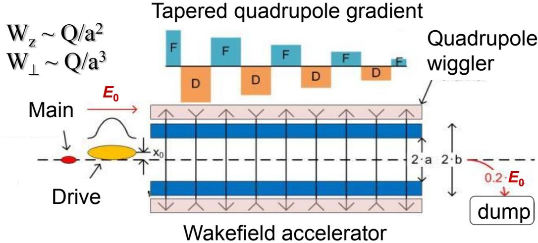
Dielectric tube with copper cladding imbedded into quadrupole wiggler
