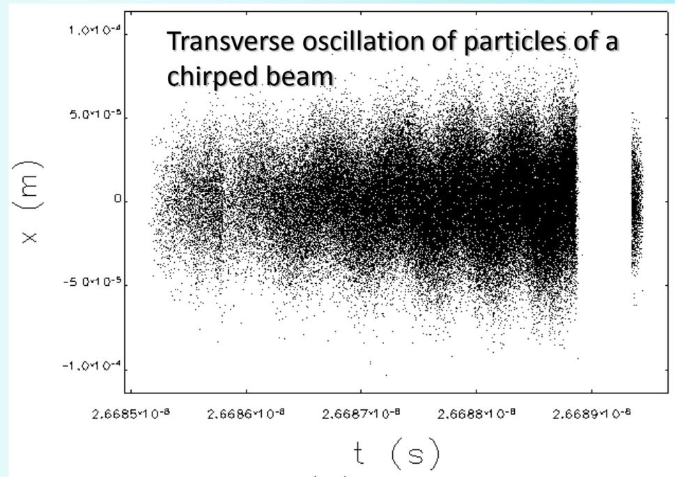
Particles of different energies have different oscillation periods in the FODO lattice
