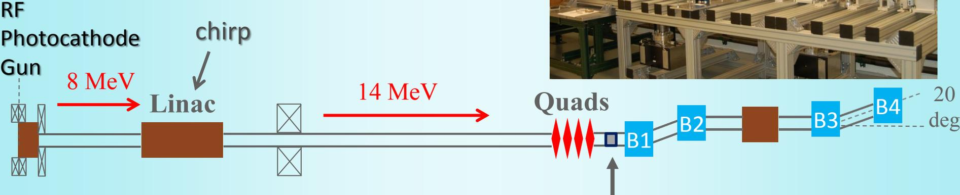
Multiple masks on motorized actuator will be used to study the bunch shaping capability of the dog-leg type EEX beamline
