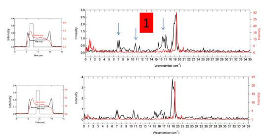
spontaneous emission using sideband generation in ZnTe and a 10 ns dye laser
