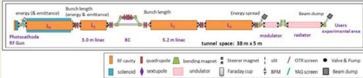
Figure 1: Layout of the proposed FEL facility at NSRRC.
