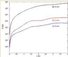
Figure 2: The growth of the radiation power in the undulator. The fundamental (66.5 nm), the 3<sup>rd</sup> harmonic (22.2 nm), and the 5<sup>th</sup> harmonic (13.3 nm) radiations are marked as black, red and blue lines, respectively.
