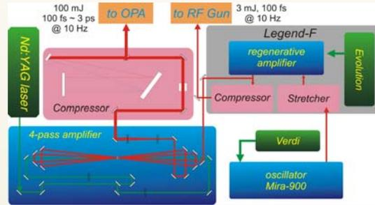
Figure 3: Layout of the upgraded laser system.
