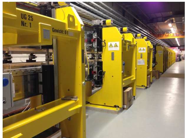
Figure 3: FLASH2 undulator beamline with twelve variable gap undulators.
