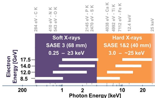
Figure 1: Photon energy reach of the two undulator types of the European XFEL at different electron energies.
