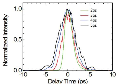
Figure 5: Pulse length measurement using cross correlation method.
