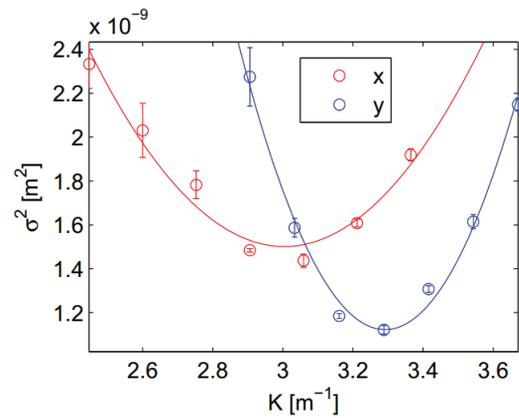
Figure 13: An example of single quadrupole scan for projected emittance measurement. Current of the third quadrupole was scanned and the beam image was measured with the screen 2.6 m downstream.
