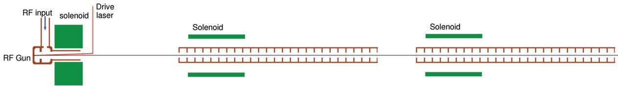
Figure 3: ITF accelerator layout with the gun and two accelerating structures.
