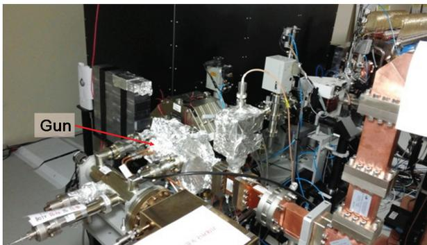
Figure 4: RF gun installed in the ITF tunnel.
