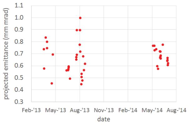
Figure 15: Projected emittance (95% rms) measured with 200 pC beams at ITF from early 2013 to summer 2014.
