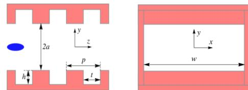
Figure 1: A flat geometry corrugated structure.
