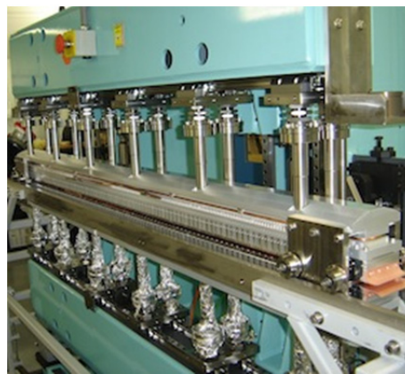
Figure 7: Example of SOLEIL U20 in-vacuum undulator.
