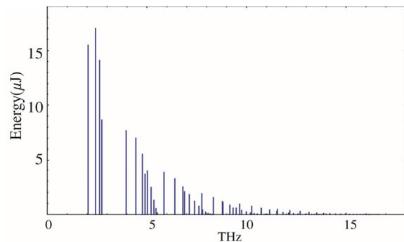
Figure 6: Discrete radiation energy spectrum for helical undulator.
