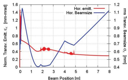
Figure 2: Transverse normalized emittance and beam size along the linac.
