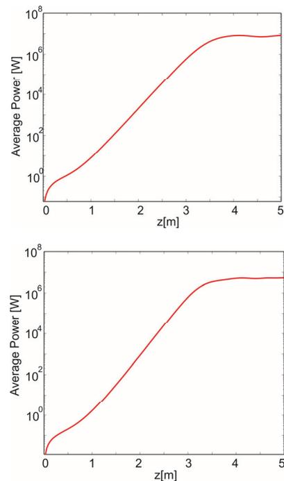
Figure 3: Average FEL power at 10  $\mu\text{m}$  (top) and 30  $\mu\text{m}$  (bottom) radiation wavelengths.
