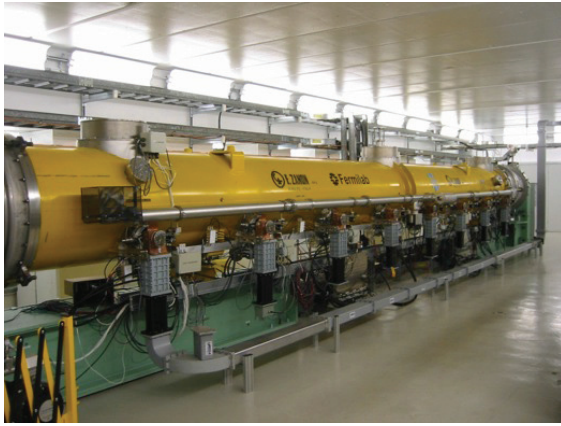
Figure 8: Cryomodule as installed in the ASTA tunnel before the waveguide distribution system was installed.
