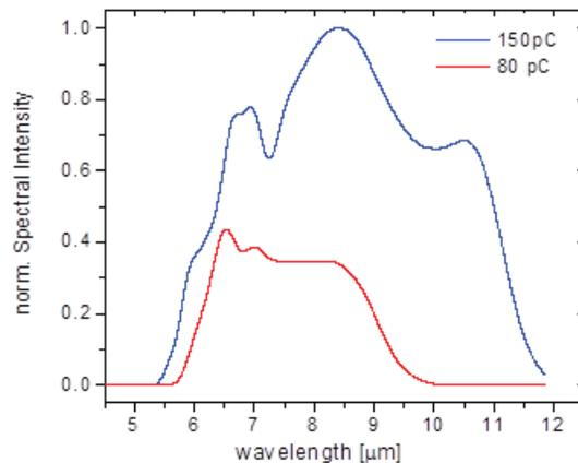
Figure 4: Pulse spectrum at saturation for 80 pC and 150 pC bunch charges.
