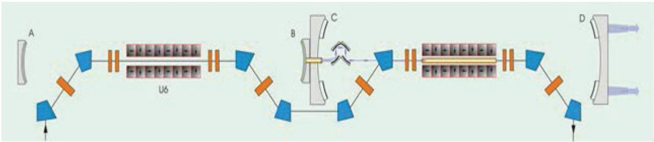
Figure 6: Schematic layout of the coupled injection-locked FEL cavities. By adjusting the settings of the resonator and the undulator modules in the respective cavities (basically cavity loss and slippage) the contribution arising from the injection locked FEL to the circulating power in the amplifier cavity can be varied. Note that the shown components are not scaled.
