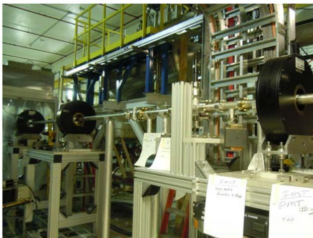
Figure 8: Solenoids and the vacuum chamber in the low-energy drift section. On the left side there is a portable clean room used for the particle free assembly. On the background the quiet helium source for the 112 MHz gun is placed on a platform
