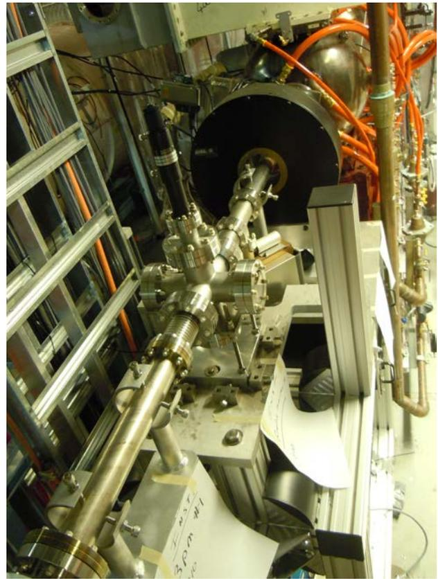
Figure 6: View of the vacuum cross with flag installed into the low energy beamline. The GigE camera will be added soon.
