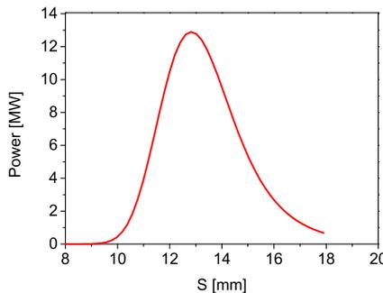
Figure 4: The radiation profile of the THz-FEL after 300 passes is shown
