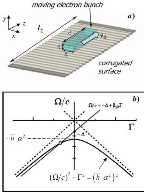
Figure 1: **(a)** Principal scheme of generation of SR pulses by an extended electron bunch moving over a periodically corrugated surface. **(b)** The dispersion diagram of the normal surface wave and resonance point in the case of a relativistic rectilinear electron beam.
