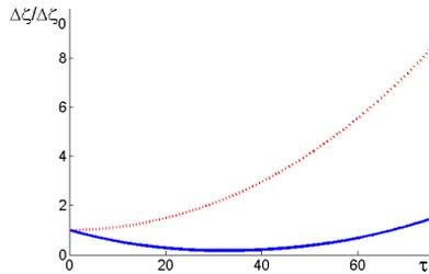
Figure 3: Change in the normalized pulse length of a moving layer with the surface density  $\sigma_0$  and initial duration 0.3 ps (uniform initial charge distribution; red - without energy chirp, blue -  $\Delta\gamma_0 = 2.7$ ).
