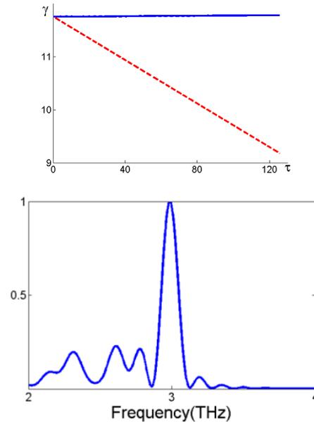
Figure 2: The Lorentz-factors and radiation spectrum for two planes with space charge parameters  $q_1$  (blue) and  $q_2$  (red). Coulomb acceleration of the front plane in the field of the rear one is compensated by the radiation deceleration.
