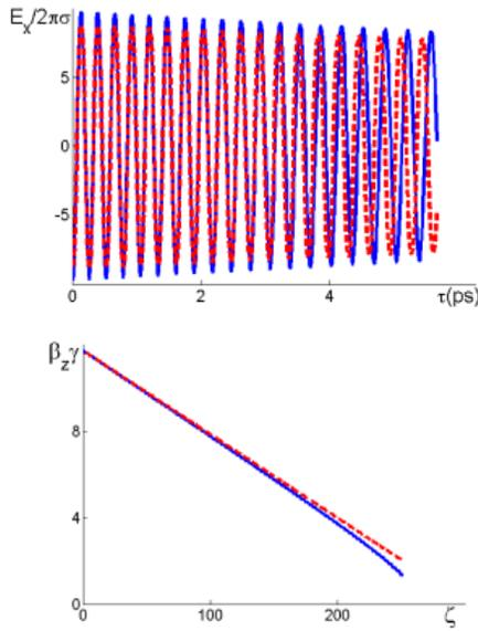
Figure 1: Radiation pulse (a) and electron axial momentum (b) for one plane: analytical (blue) and numerical (red) solutions.
