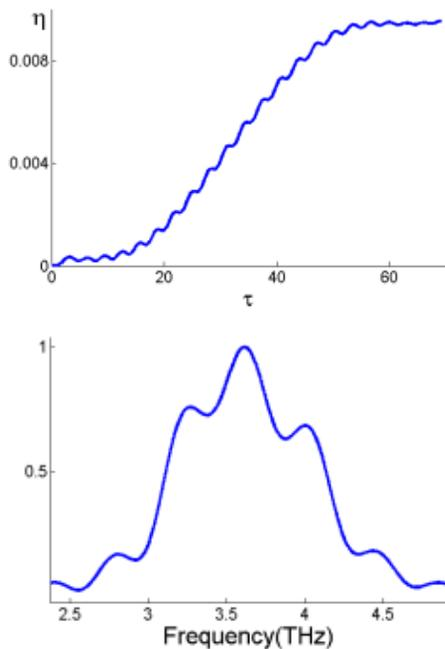
Figure 4: Current efficiency and radiation spectrum for a moving layer with initial duration 0.3 ps.
