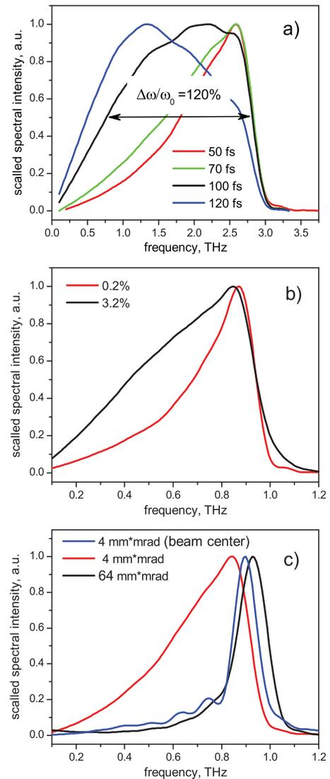
Figure 3: (Color online) The scaled output spectra calculated for different bunch durations at  $f_R=3.0$  THz,  $\delta=1\%$ , and  $\epsilon_n=4$  mm·mrad (a); for two  $\delta$  values at  $f_R=1.0$  THz and  $\epsilon_n=8$  mm·mrad (b); for two  $\epsilon_n$  values at  $f_R=1.0$  THz and  $\delta=1\%$  (c).
