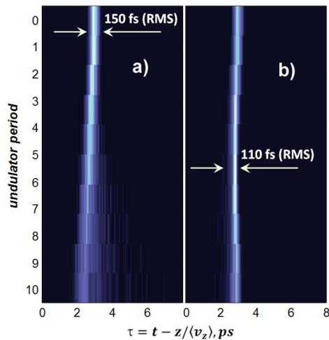
Figure 2: (Color online) The density maps of electron trajectories in a coasting frame calculated for  $\epsilon_n=64$  mm·mrad (a) and  $\epsilon_n=4$  mm·mrad (b) when  $\delta=1\%$  and  $f_R=1.0$  THz.
