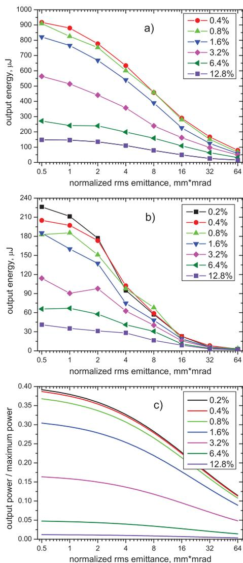
Figure 1: (Color online) The output energy of THz pulses as a function of  $\epsilon_n$  for different  $\delta$ -values at  $f_R=0.3$  THz (a) and  $f_R=3.0$  THz (b). The relative THz power is analytically evaluated for  $f_R=3.0$  THz (c).
