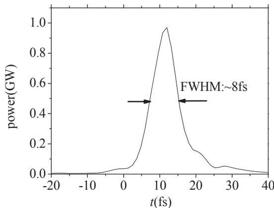
Figure 5: Pulse structure of 30 nm radiation. The pulse length is 8 fs (FWHM).
