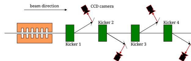
Figure 1: Generic layout of a slice emittance monitor.
