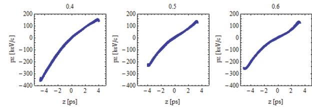
Figure 8: Longitudinal phase space of a 250 pC bunch at the exit of the CLARA first linac for gun first cell lengths marked above, for a gun peak field of 100 MV/m.
