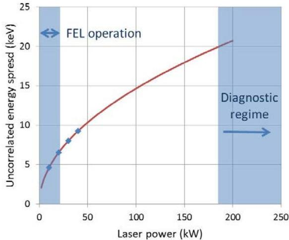
Figure 13: RMS uncorrelated energy spread versus Laser power. Blue dots from Elegant simulations assuming 150 MeV, 1040 nm laser wavelength, 400 μm laser waist, read equation 2.
