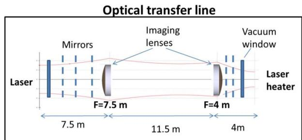
Figure 7: Schematic of the laser transfer line.
