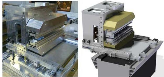
Figure 12: U50 during assembly at Daresbury Laboratory and 3D model of the undulator on the support girder in extracted position.
