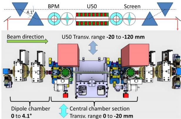
Figure 4: Movable parts in the LH chicane, with undulator in retracted position and chicane at 4.1°.
