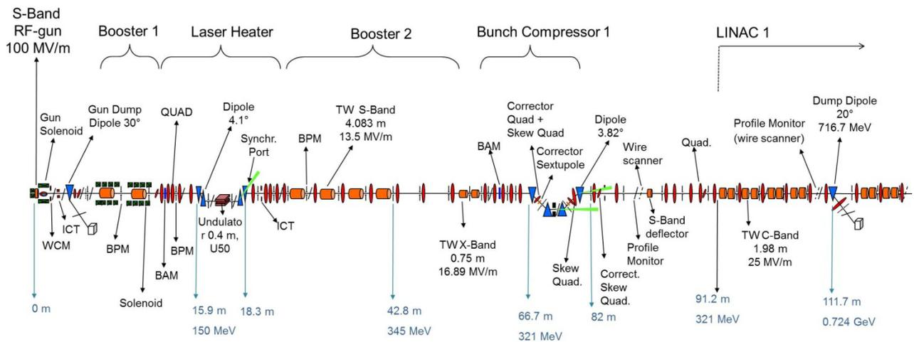
Figure 1: SwissFEL injector facility, schematic layout.
