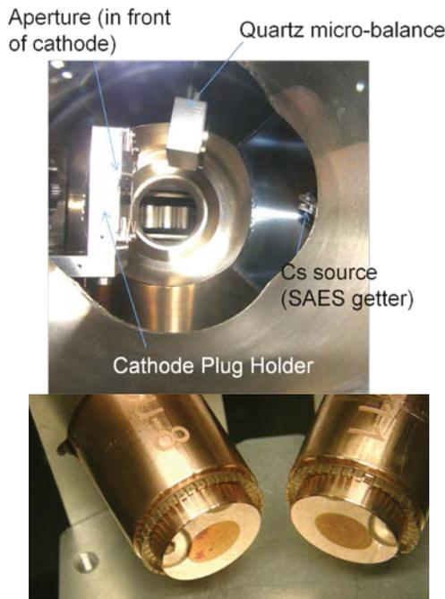
Figure 2: Evaporation chamber with the cathode holder and micro balance on the left and the Cs evaporation source on the right. (Top); Two cathodes with a 1 cm diameter disc of Cs<sub>2</sub>Te (Bottom).
