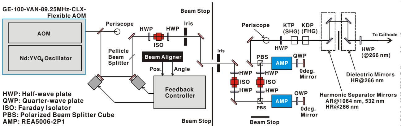
Figure 2: Configuration of photocathode drive laser system.
