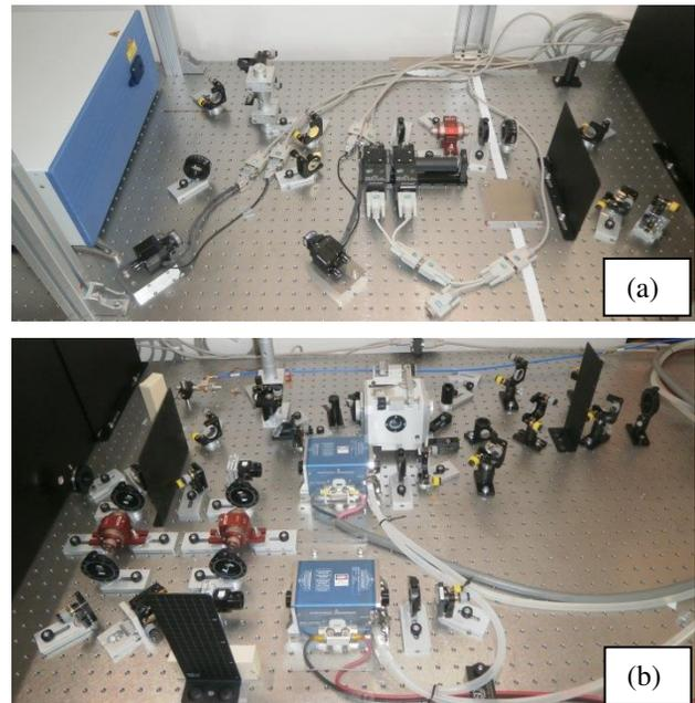
Figure 1: Photographs of the developed drive laser system. (a) Upstream side including the Nd-YVO<sub>4</sub> oscillator and the beam alignment feedback system. (b) Downstream side including the double-pass amplifiers and harmonic generation crystals.
