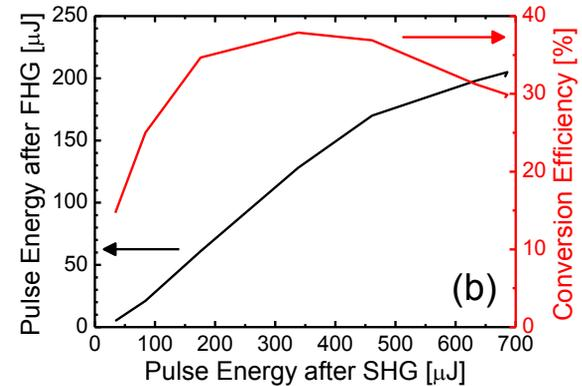
Figure 4: Laser pulse energy after SHG and FHG plotted with their conversion efficiencies as a function of incident laser pulse energy to the crystals. (a) Pulse energy after SHG and conversion efficiency of SHG. (b) Pulse energy after FHG and conversion efficiency of FHG.
