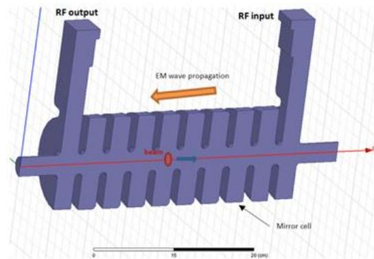
Figure 1: Schematic diagram of Transverse RF Deflecting Cavity.
