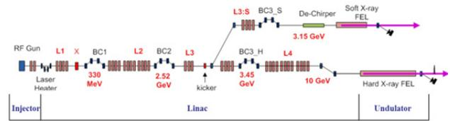
Figure 1: Schematic diagram of PAL-XFEL. The SX branch line is on the middle of the linac lattice.
