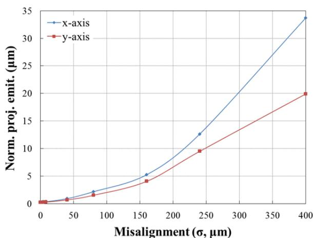
Figure 4: The emittance dilution by misalignments of all elements in the linac lattice.
