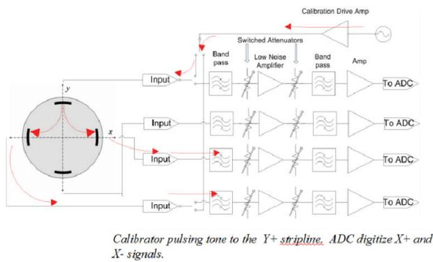
Figure 3: Stripline BPM front end electronics.
