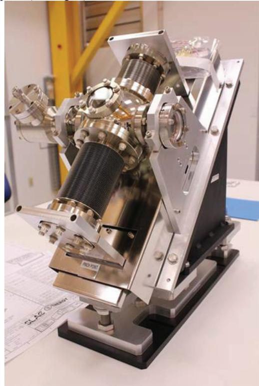
Figure 7: Fast wire scanner tested at SLAC.
