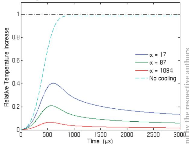
Figure 8: Wire temperature rise (normalized) as a function of wire thermal diffusion in mm<sup>2</sup>/sec.
