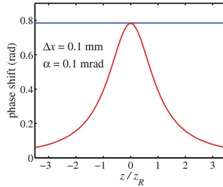
Figure 4: Phase shift of energy modulation for a transverse displacement of  $\Delta x = 0.1$  mm and a wavefront tilt angle of  $\alpha = 0.1$  mrad as function of longitudinal coordinate  $z$ , normalized to the Rayleigh length  $z_R$ , for the case of a plane wave (blue) and a Gaussian laser waist at  $z = 0$  (red).
