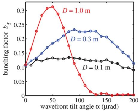
Figure 3: Bunching factors calculated for CHG at the 5th harmonic with the beam parameters of DELTA and different values of dispersion  $D$  at the modulator. The laser field is assumed to consist of plane waves arriving under a tilt angle  $\alpha$  with respect to the electron beam.
