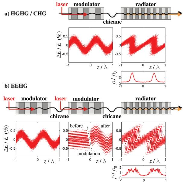
Figure 1: Setup for seeding schemes: a) HHG or CHG and b) EEHG with respective electron distributions in phase space, i.e. longitudinal coordinate  $z$ , here normalized to the laser wavelength  $\lambda$ , versus relative energy deviation  $\Delta E/E$ .
