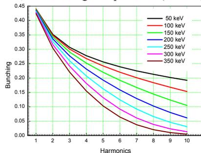
Figure 2: Bunching factor for HGHG with different initial slice energy spreads.
