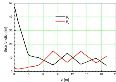
Figure 5: Betatron function in the seeding undulator section.
