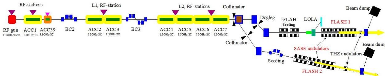
Figure 1: Schematic layout of FLASH facility.
