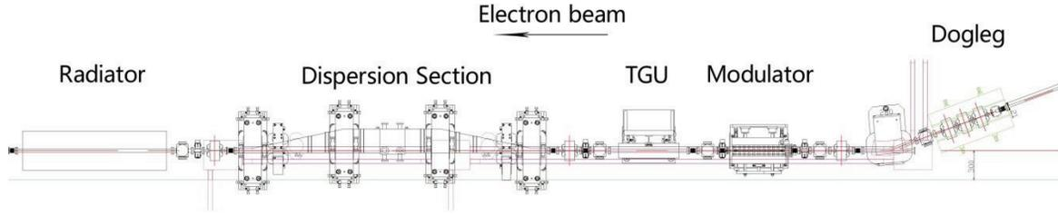
Figure 2: Layout for the PEHG experiment at SDUV-FEL.
