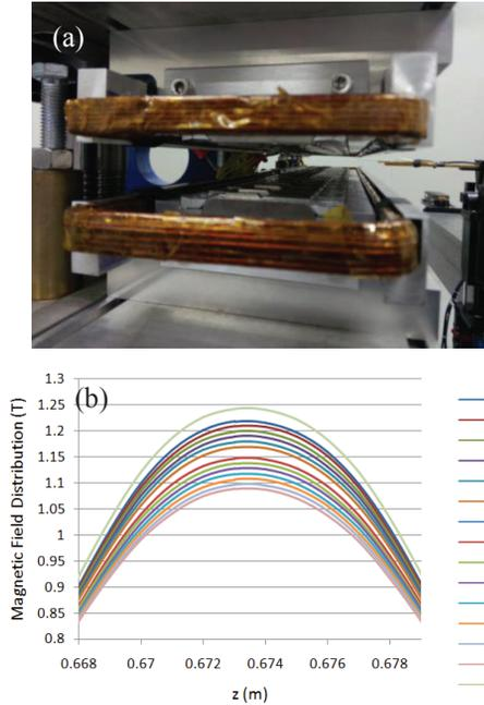
Figure 3: (a) The TGU for PEHG experiment. (b) Measurement results of magnetic field distributions for different transverse position of TGU.
