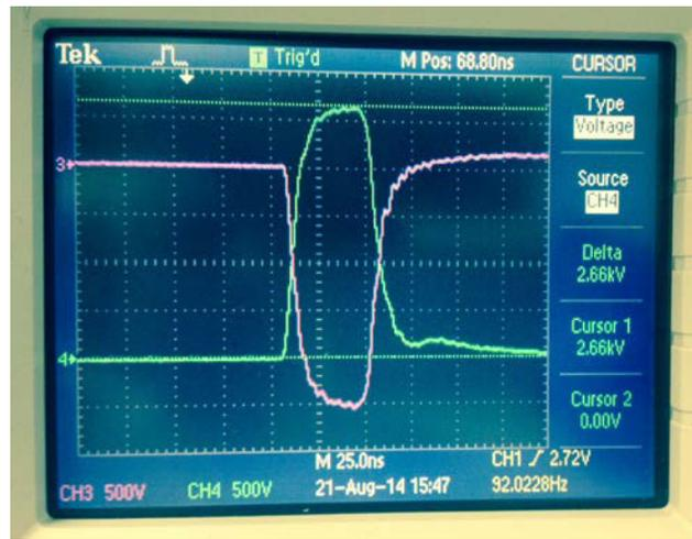
Figure 3: Output of two boards into 100 ohms operating in bipolar mode. 5 kV (+/- 2.5 kV), 5 ns 10 – 90% risetime, 25 ns pulsewidth.
