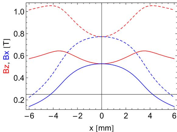
Figure 5: Transverse variation of the peak fields in inclined and circular (dashed) mode. The good field region of  $10^{-4}$  is  $50\mu\text{m}$  for the vertical field and  $60\text{-}80\mu\text{m}$  for the horizontal.
