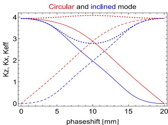
Figure 6: Shift dependent variation of  $K_z$  (solid),  $K_x$  (dashed) and  $K_{\text{eff}}$  (dotted) for circular and inclined polarization. The  $45^\circ$  magnetization and slit =  $\text{gap}_{\text{min}}$  result in this symmetric plot.
