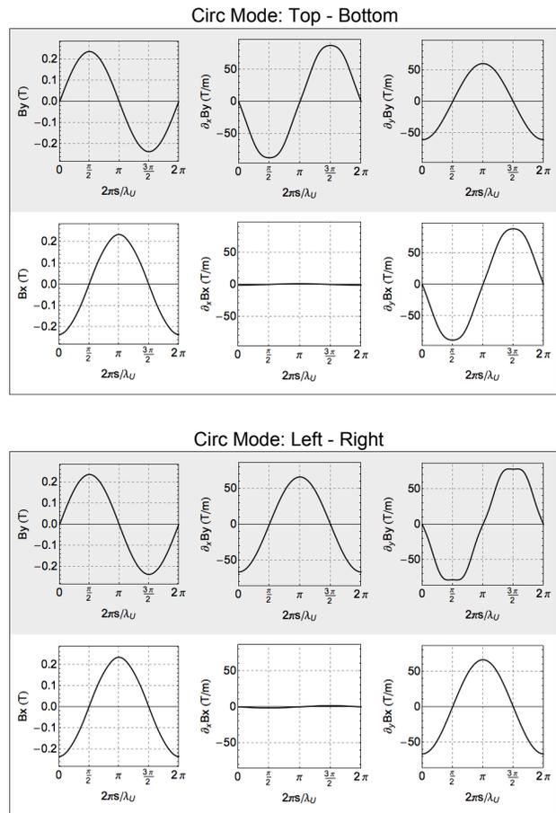
Figure 7: Field gradients in fixed gap APPLE operation with energy shift in Top - Bottom and Left - Right configuration.
