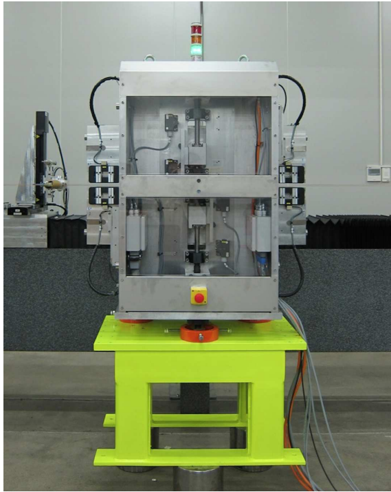
Figure 2: Linear polarization undulator, manufactured by Kyma s.r.l.
