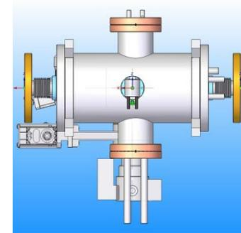
Foil-based backscattering monitor
